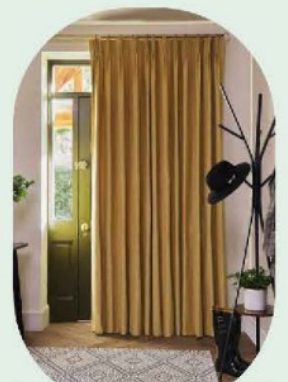
Adding rugs to hard flooring, and heavy curtains in front of doors and windows, can help to absorb sound.
